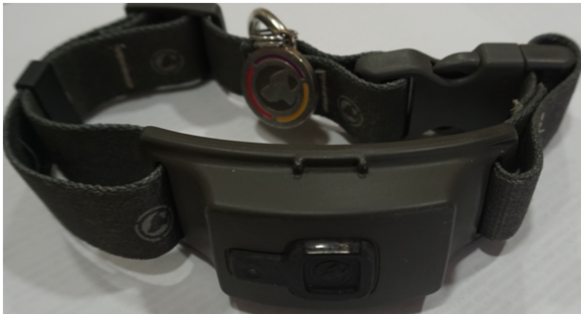
Figure 2. Voyce Health Monitor™ size medium with emphasis on the plastic box that contains the accelerometer component.
